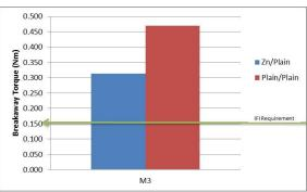
Electroloc<sup>TM</sup> meets or exceeds the requirements of the IFI-525 (2007) specification. Results for 24 hour cure at ambient temperature are shown above. While results are shown for small fasteners, Electroloc<sup>TM</sup> is not limited to use on these sizes.
