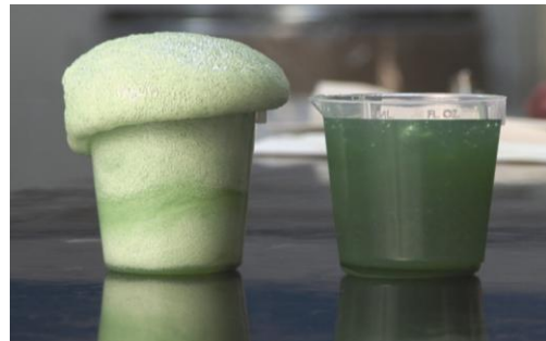
As shown in this Laboratory Demonstration, ND Expand-A-Seal expands volumetrically 20-50%
