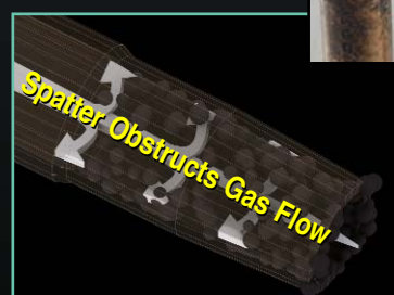
Inferior, Porous Weld
